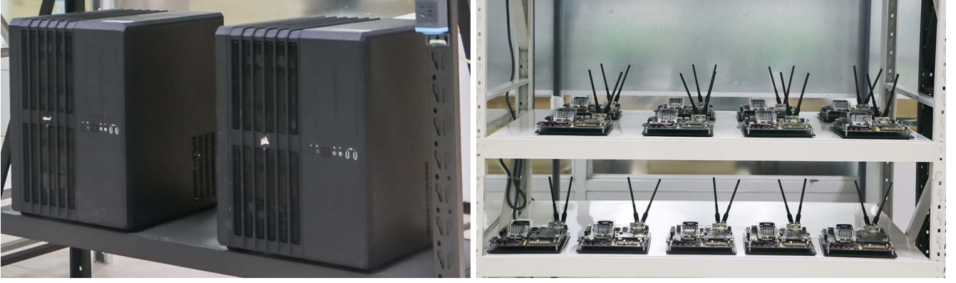
Fig. 3. Hardware devices of our testbed. Left : Parameter Server; Right : TX2.
